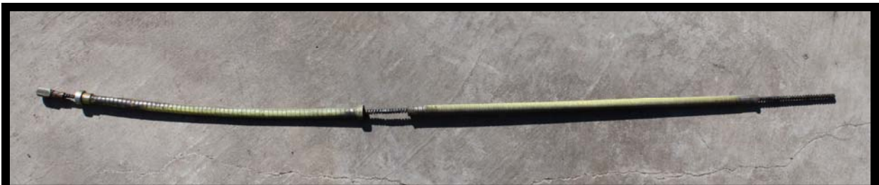
George Mocabee worked on his Mets windshield wipers. Below is the windshield wiper cable in its armor, which George took out and later cleaned and reinstalled.
