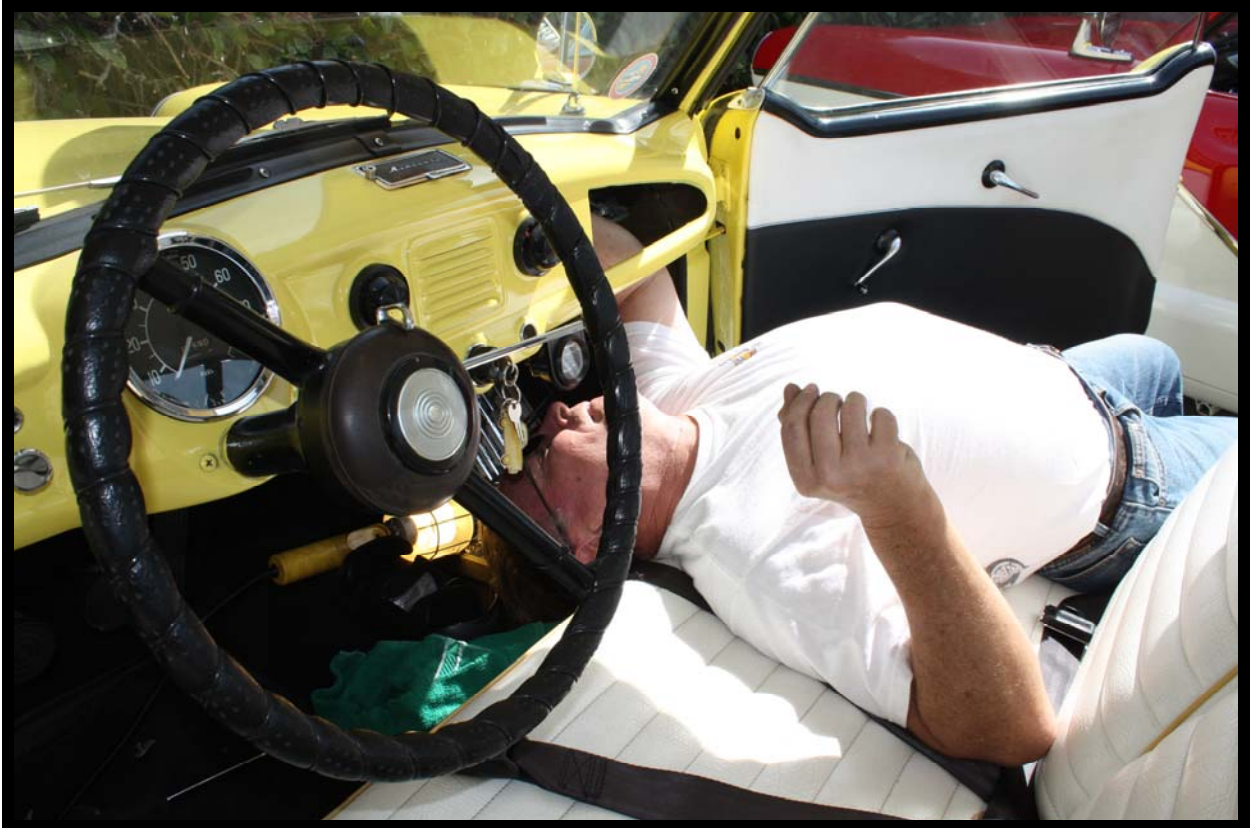
George Mocabee worked on his Mets windshield wipers. Below is the windshield wiper cable in its armor, which George took out and later cleaned and reinstalled.
