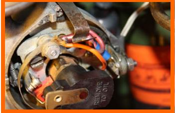
It wasn't too broken so I fixed it and broke it better! My Met was getting to the point where it hesitated when I accelerated from a slow RPM. High RPM was fine. It was suggested to me that the distributor points were possibly too close together. Another suggestion was that the accelerator pump in the carburetor needed attention.
